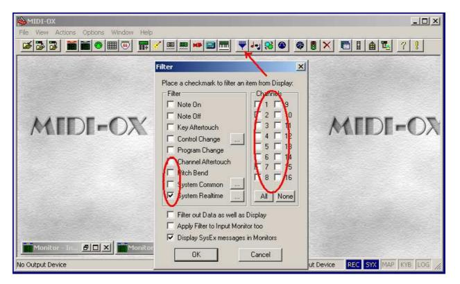
System Realtime and System Common are most likely to be the messages we don't want to see. Experiment with settings for your system to get the minimal view required. Also see extra settings under the "..." buttons.
